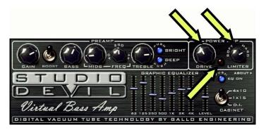
The POWER AMP / LIMITER controls allow you to add compression and loudness to your sound while minimizing the amount of harsh distortion and audible clipping, just like when you turn up the volume on a real amp. Here's how the controls work:
